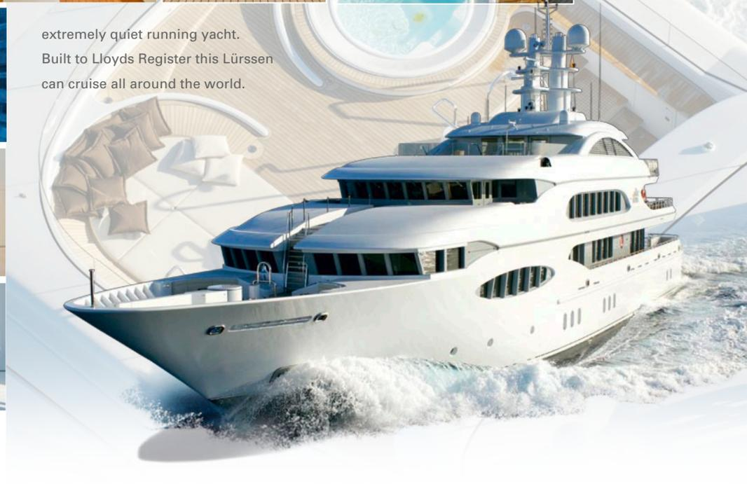
Powered by two Caterpillar engines of 1,455 kW each, she reaches a top speed of 15,5 knots and has a range of 7.000 nm. Advanced sound and vibration features guarantee an
