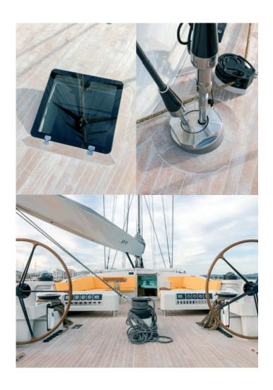
Built by the Shipyard C.N.B. in Bordeaux, this very modern sailing yacht was launched in june 2009. Designed for offshore sailing, her owner is an experienced yachtsman who requested a sensitive vessel which is pleasant to sail. The rigging and mast are made from carbon and the sails in kevlar which increases her draft from 2 to 4m.
