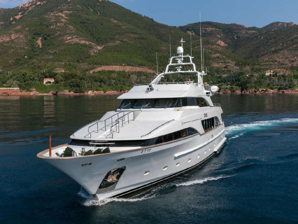
Built with a GRP hull and superstructure, she benefits from a semi-displacement hull to provide exceptional seakeeping and impressive speeds. Powered by twin Caterpillar engines, she comfortably cruises at 12 knots in fuel economy and reaches a maximum speed of 15 knots with a cruising range of up to 3,200 nautical miles. An onboard stabilization system ensures comfort when underway.
