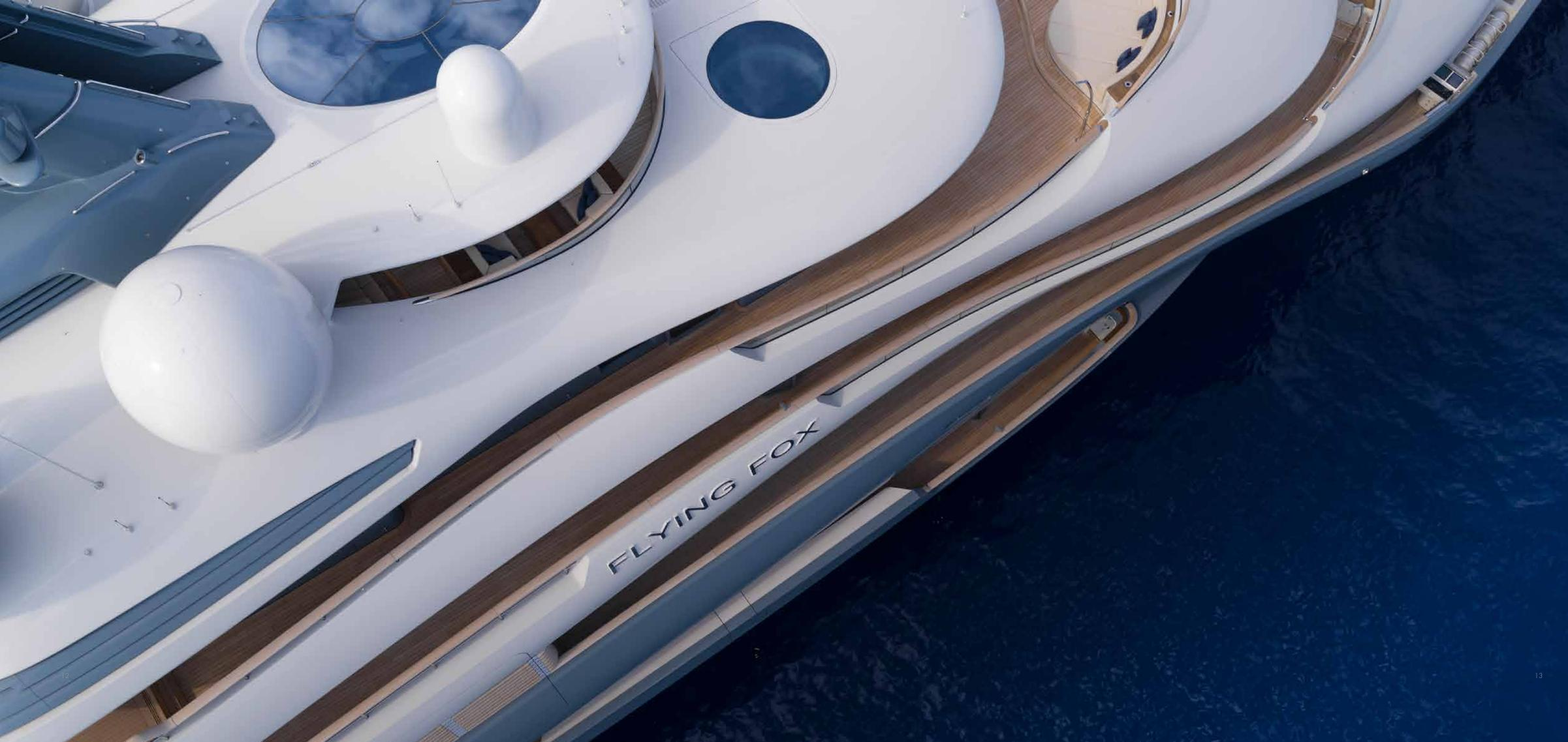
LYING FOX is built with a steel hull and an aluminium superstructure. The shapely curves proved an enormous, yet satisfying, challenge for the welders. Perhaps even more amazing is her performance: FLYING FOX is capable of 20 knots flat, with a cruising speed of 15 knots.
